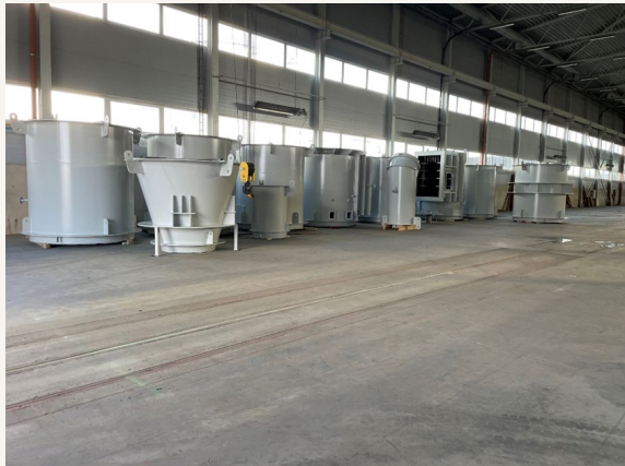
Reactor parts ready for refractory works
