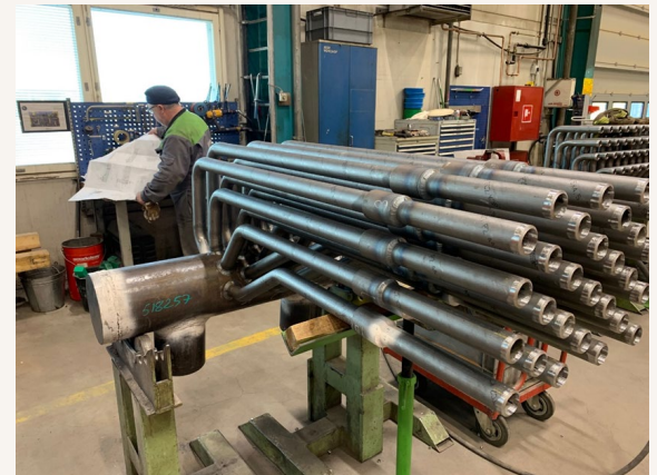
Loopseal evaporator header and tubes
